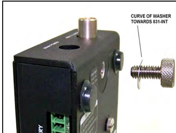
**FIGURE 2-13 Placement of Stainless Steel Mounting Hardware**
