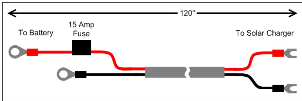
**FIGURE 2-8 CBL161 Cable 100 AH Battery to Solar Charger**
